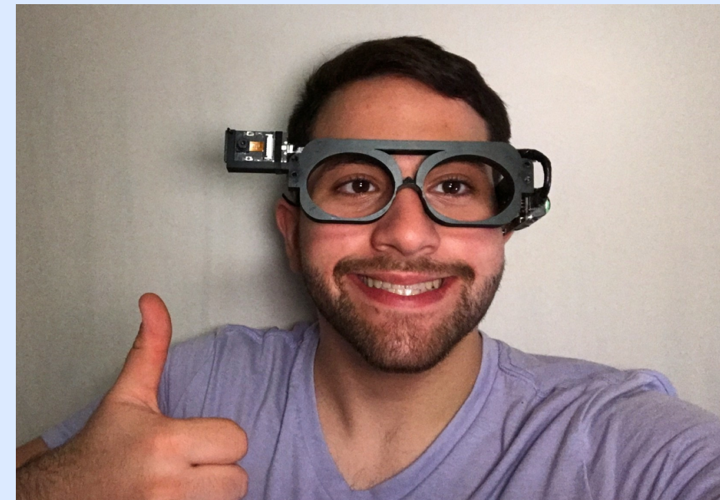
Figure 1: 3D printed glasses with ESP-EYE and battery-shield mounted
